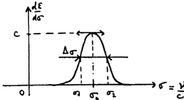
$$\frac{d\mathcal{E}}{d\sigma} = f(\sigma) = C \exp\left[-\frac{(\sigma - \sigma_0)^2}{a^2}\right] \quad : \quad \text{profil Gaussien}$$
